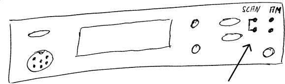
Please open this jumper and solder a new jumper into the holes named "AM"
